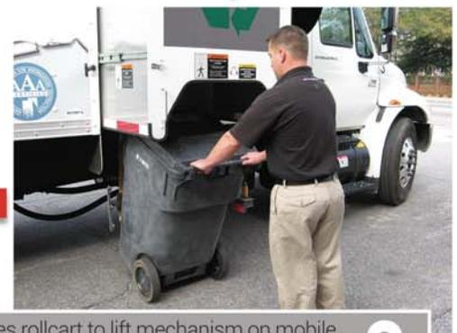
CSR attaches rollcart to lift mechanism on mobile shred truck which lifts and empties contents directly into on-board shredder.
